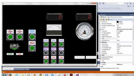
**Figure 8. Developing the HMI application using Visual Studio 2013**
