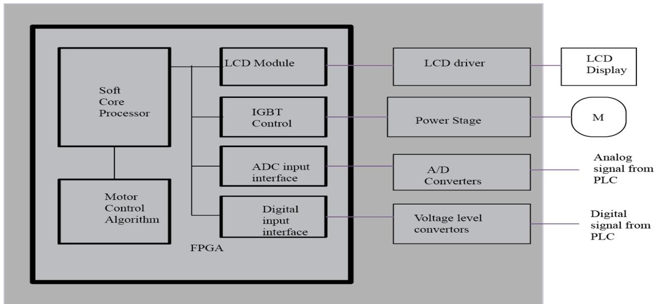
**Figure1. Block Diagram of the Designed VSD**
