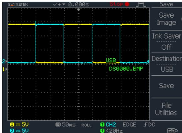
**Figure 11. Oscilloscope Trace for Gating Signals to Switching Devices of the Same Leg**
