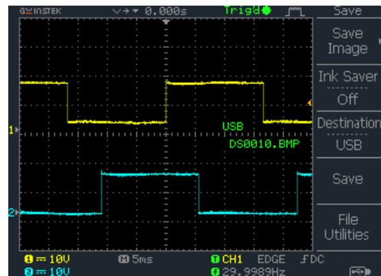
**Figure 13. Gating Signals for Two Switching Devices on Different Legs**
