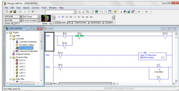
**Figure 7. Programming the PLC using RSLogix 500**
