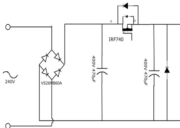
**Figure 5. Power Circuit Schematic**
