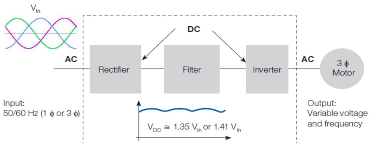
**Figure 2. Operational Diagram of the VSD**
