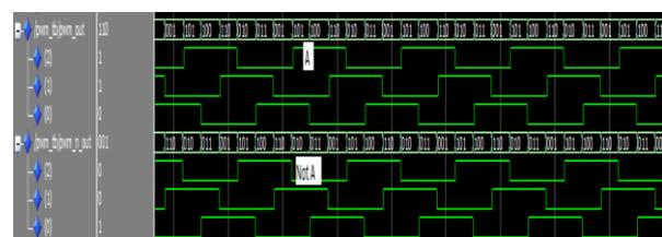
**Figure 10. Output of Simulating Three Phase PWM Signal**
