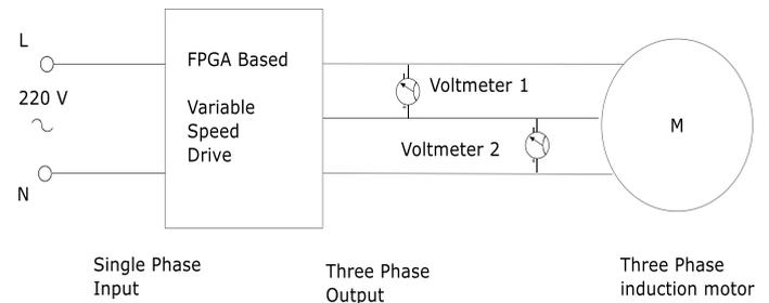
**Figure 14. Experiment to Determine variation of Voltage with Frequency**
