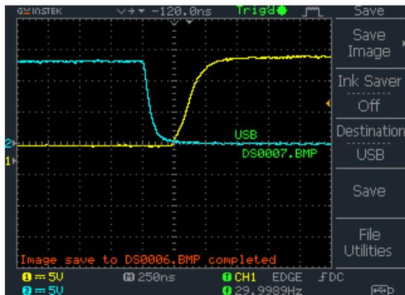
**Figure 12. Signal Showing Dead Time**
