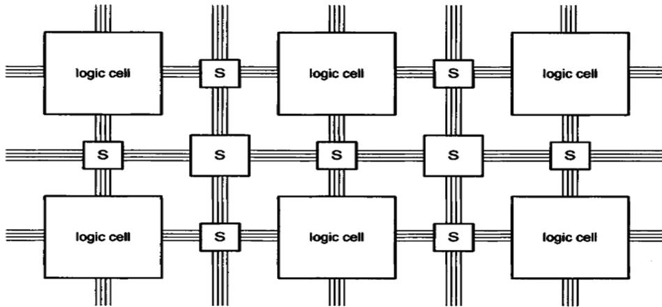
Figure 3. Structure of Altera Cyclone II FPGA Device
