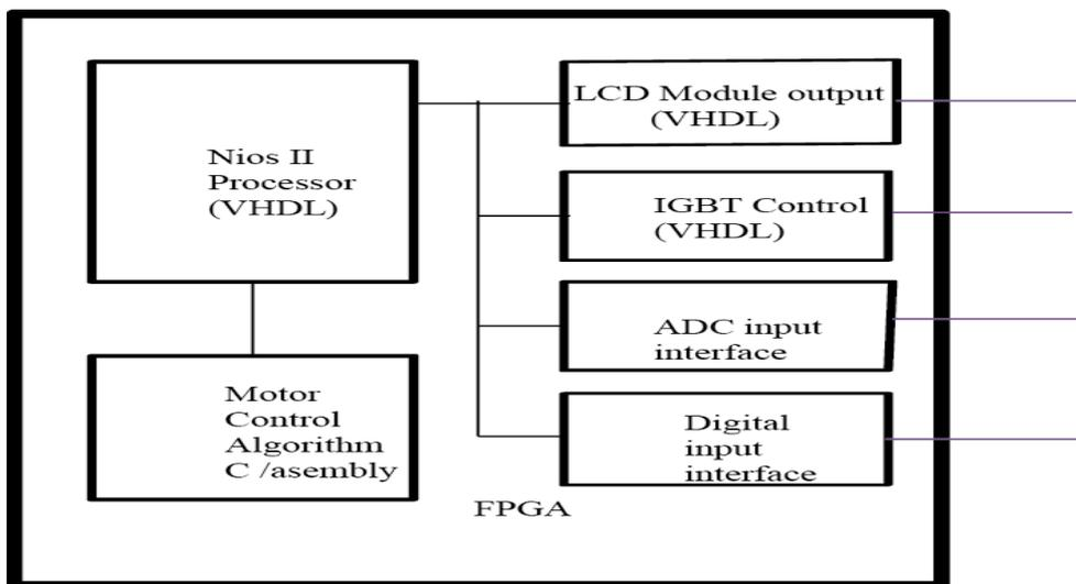
Figure 4. Proposed Blocks inside the FPGA Chip
