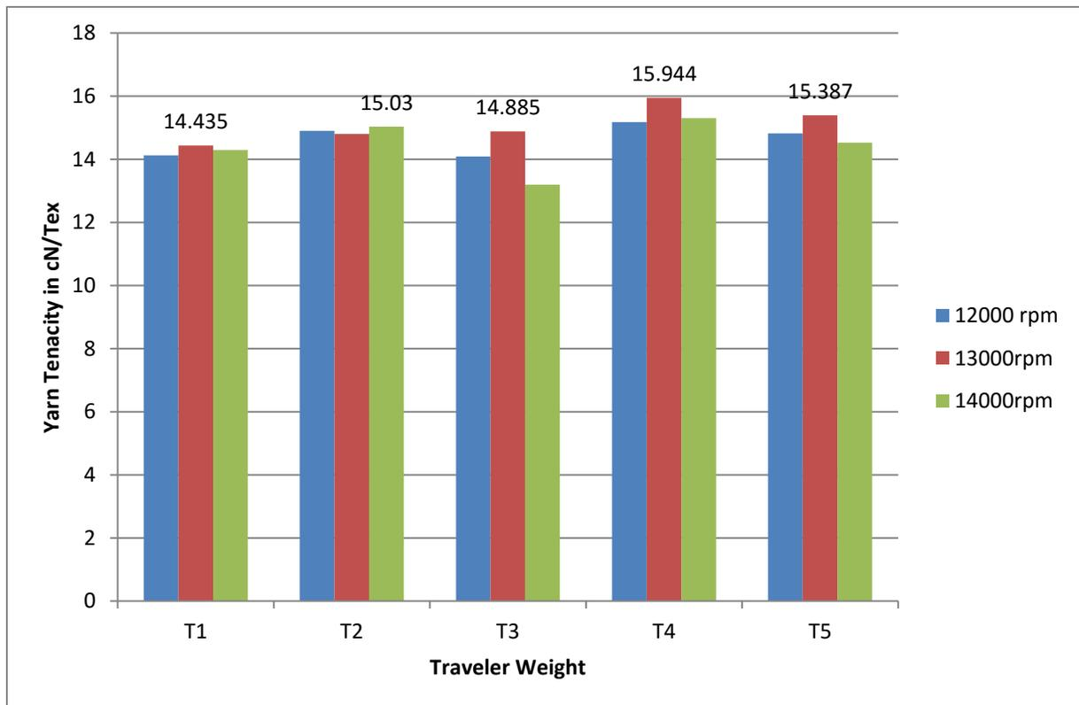
**Figure 1. Effect of Traveler weight and spindle speed on yarn tenacity**
