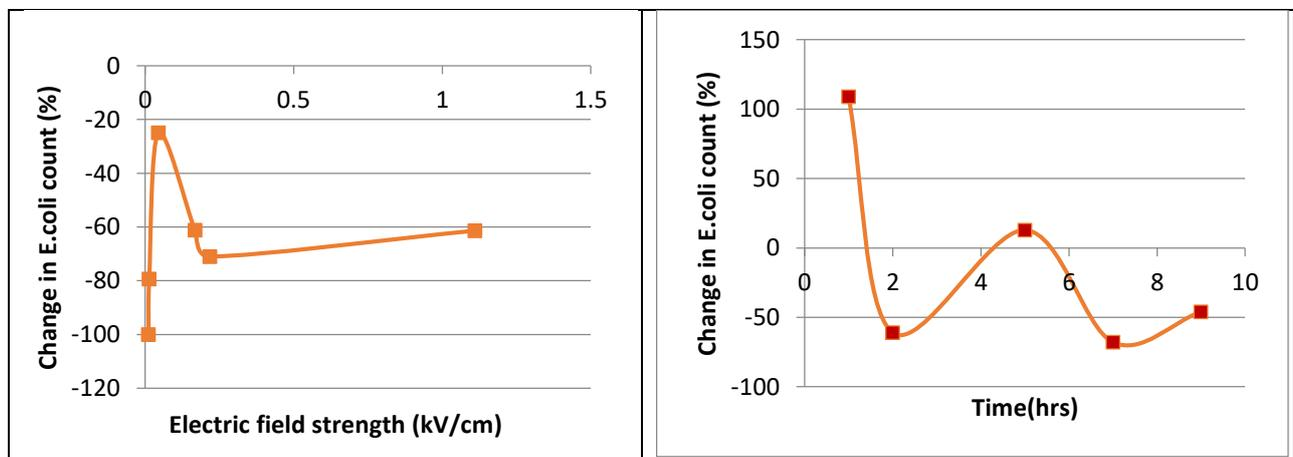
**Figure 2: The change in *E. coli* bacteria count (Vs.) exposed AC electric field for 2 hours (left panel). The electric field applied ranged from 0.011 to 1.1 kV/cm. Changes in *E. coli* bacteria count in a sample exposed in AC electric field (1 kV/cm) for different exposure periods (right panel).**
