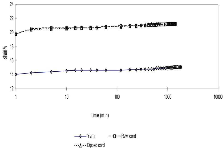
Fig 4: Creep - time relationships of yarn, raw cord and dipped cord at 75°C
