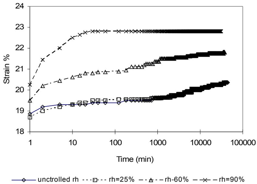
**Fig 6 Effect of humidity on creep of raw cord at 35 °C**
