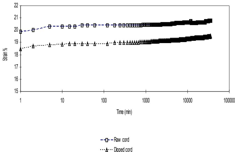
Fig 3: Creep - time relationships of raw cord and dipped cord at room temperature
