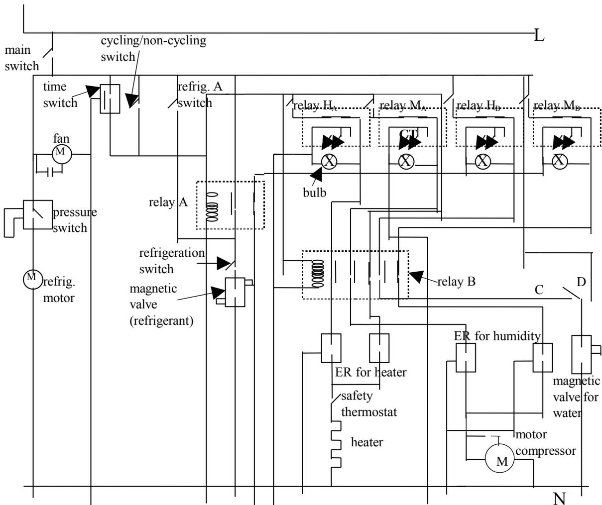
**NB:** ER are energy regulators for heater and humidity; C and D switch on main supplies to water valve
